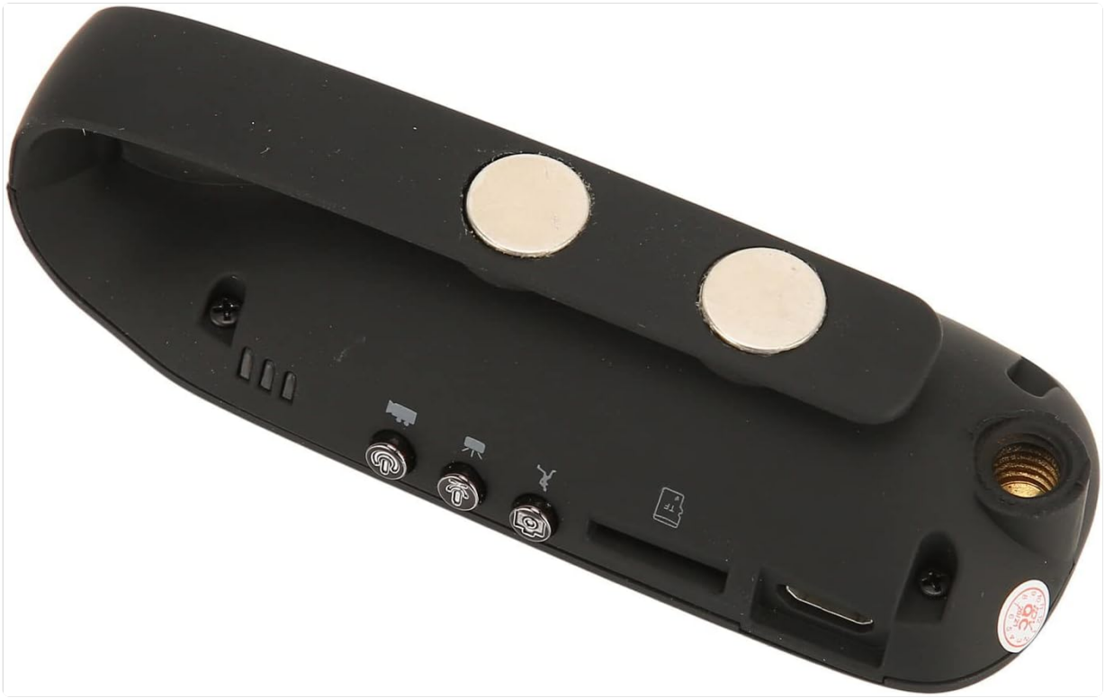
Image 2: Back view of the Elprico IDV007 Body Camera, illustrating the clip, memory card slot, and USB charging port.
