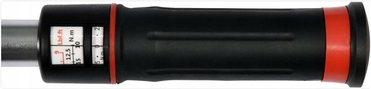
Figure 3.5: A close-up view of the torque adjustment scale located on the handle of the Yato YT-07612 torque wrench. The scale shows markings for both Nm and Lbf.ft, allowing precise setting of the desired torque.
