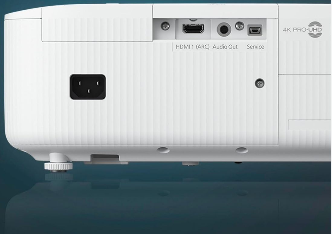
Figure 4: Rear ports of the EH-TW6250 Projector.
