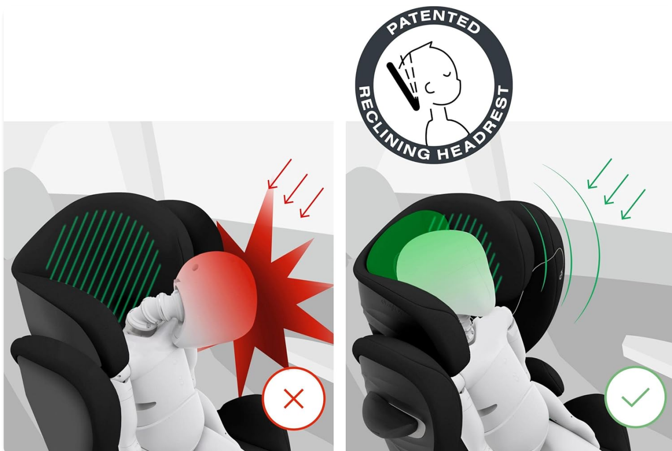
Figure 3.2: Illustration of the patented reclining headrest, showing how it keeps the child's head safely within the headrest during sleep.
