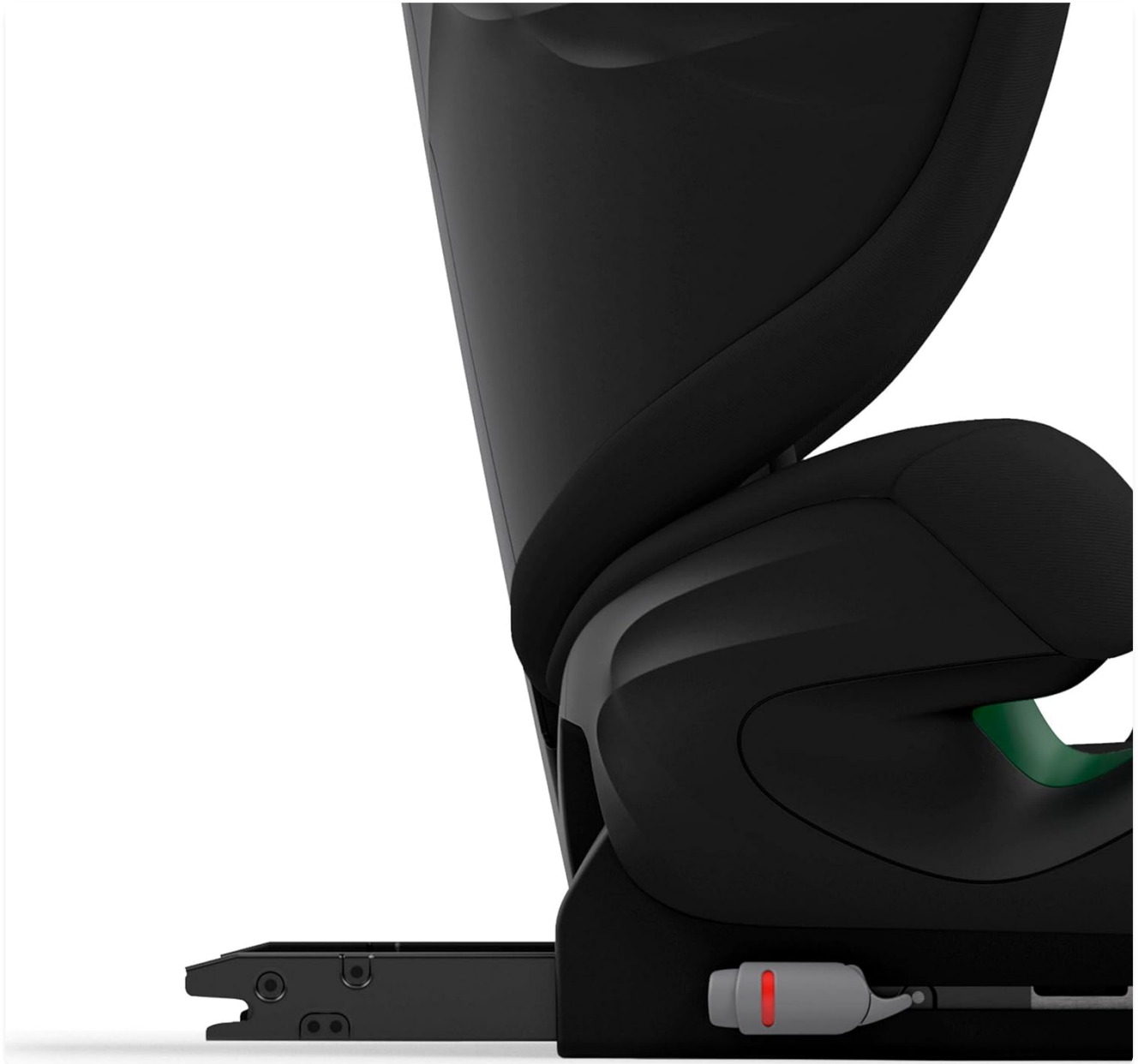
Figure 2.1: ISOFIX connectors extended from the car seat base. The red indicator shows the unlocked position, which will turn green upon correct installation.
