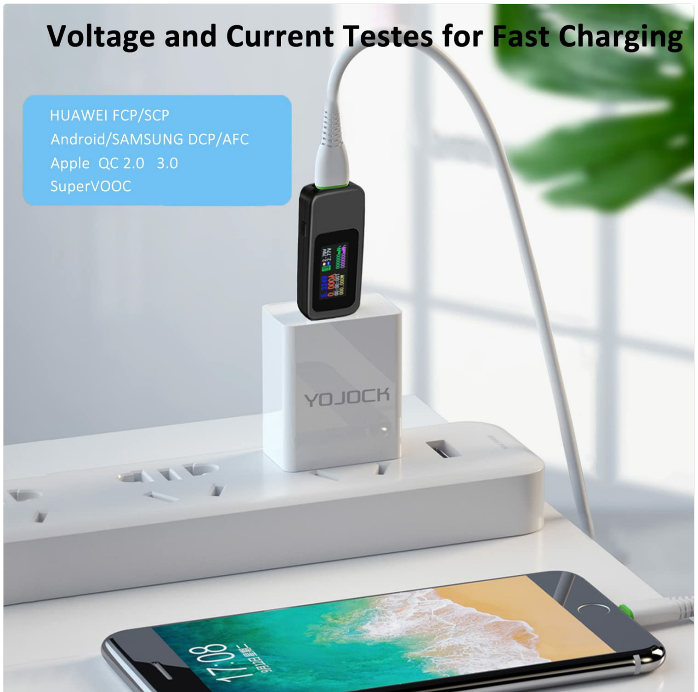
Figure 2.1: Connecting the USB tester between a charger and a device for fast charging tests.
