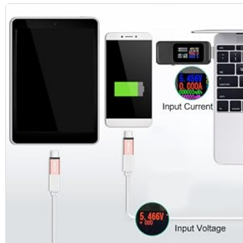
Figure 2.2: Illustration of input current and voltage measurement flow.
