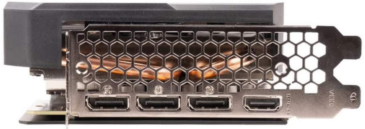
Rear I/O panel with multiple DisplayPort and HDMI outputs for display connectivity.
