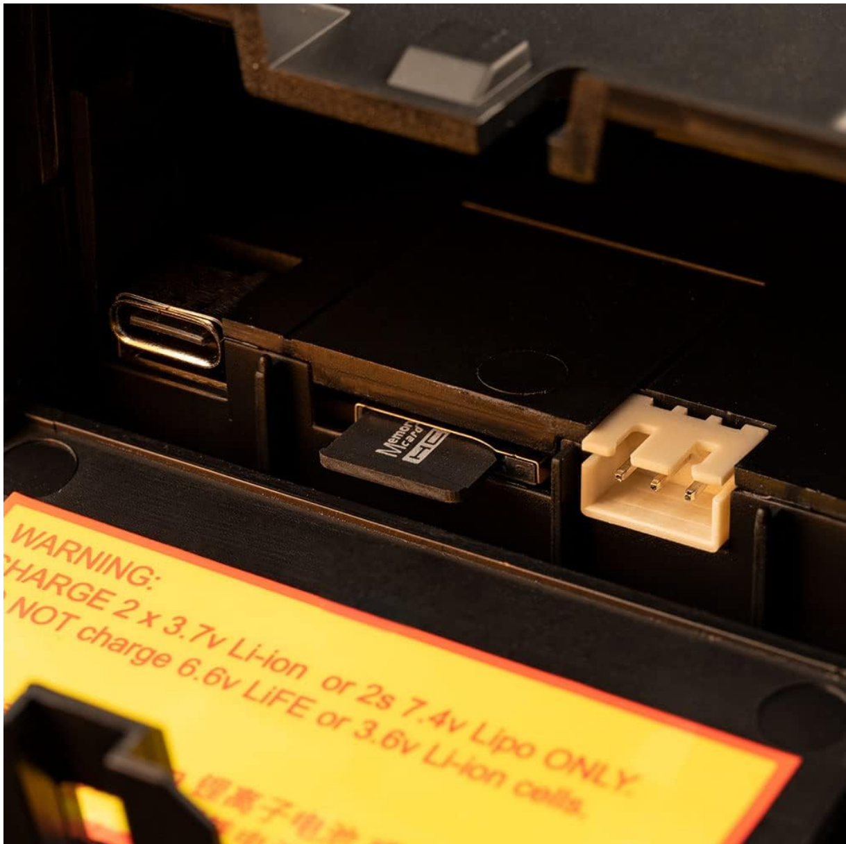
Image 4.1: A close-up view of the microSD card correctly inserted into its dedicated slot within the battery compartment.
