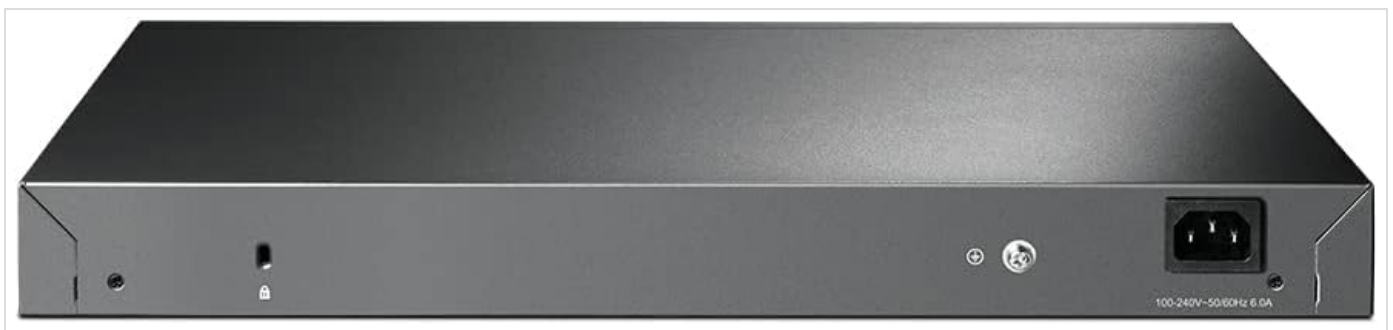
Figure 4.2: Rear view of the TP-Link TL-SG3452XP switch, displaying the power input and grounding point.
