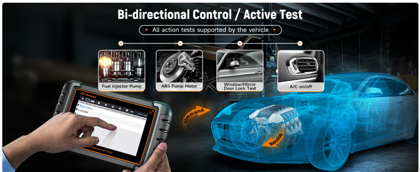
Figure 3.12: Bi-directional Control / Active Test Examples
