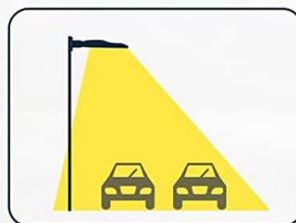
Image 6.1: Example of parking lot illumination, demonstrating Type III light distribution for wide coverage.
