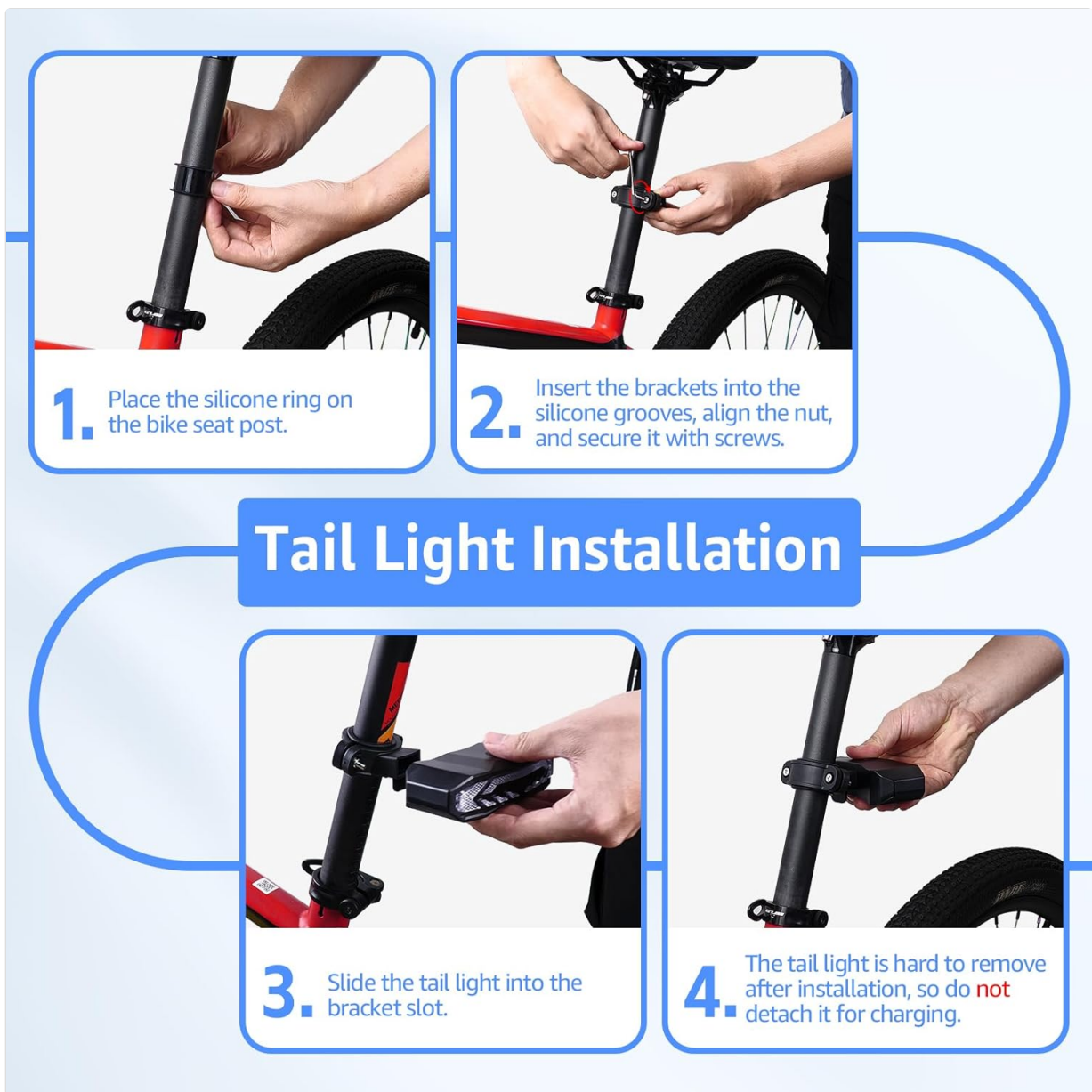
Figure 4.1: Taillight installation steps.
