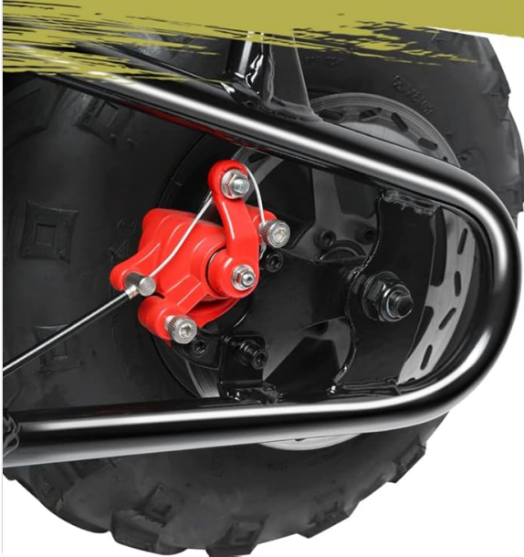
Figure 2.4: Detail of the off-road tires and rear disc brake for safety and performance.
