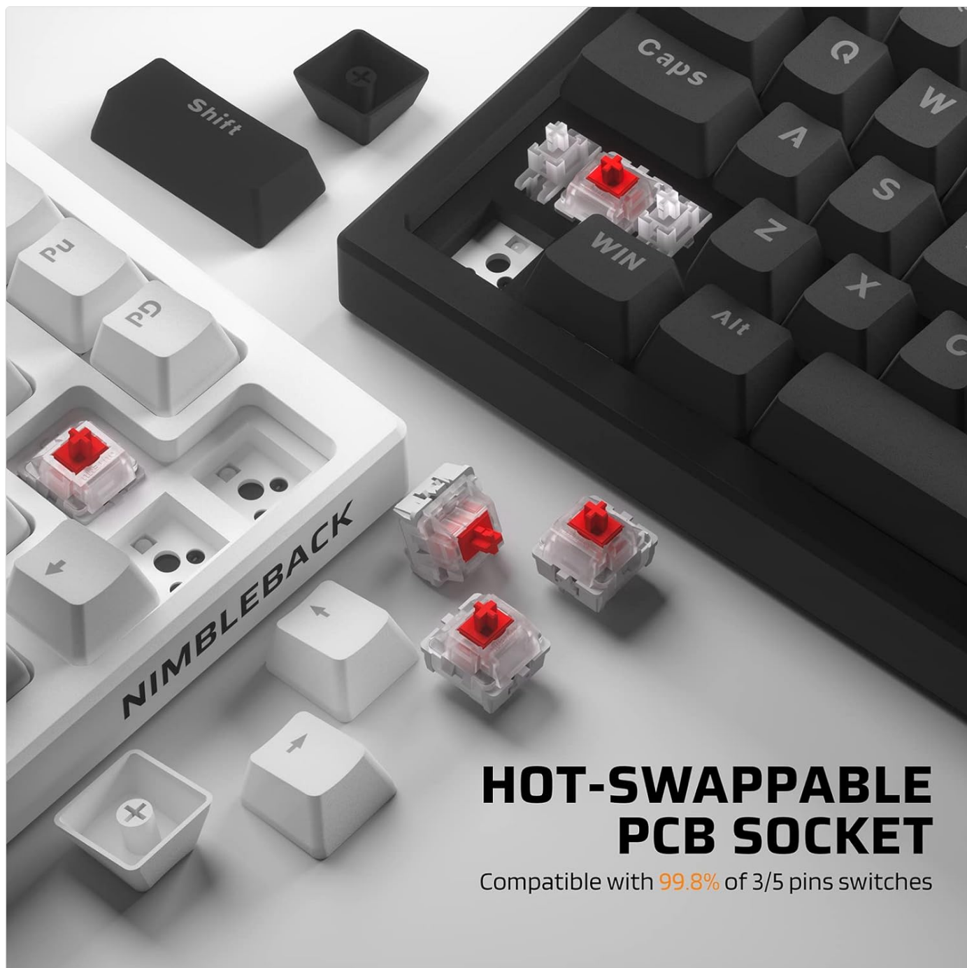
Image: Demonstrating the hot-swappable feature of the LTC Nimbleback NB831, allowing for easy switch replacement.
