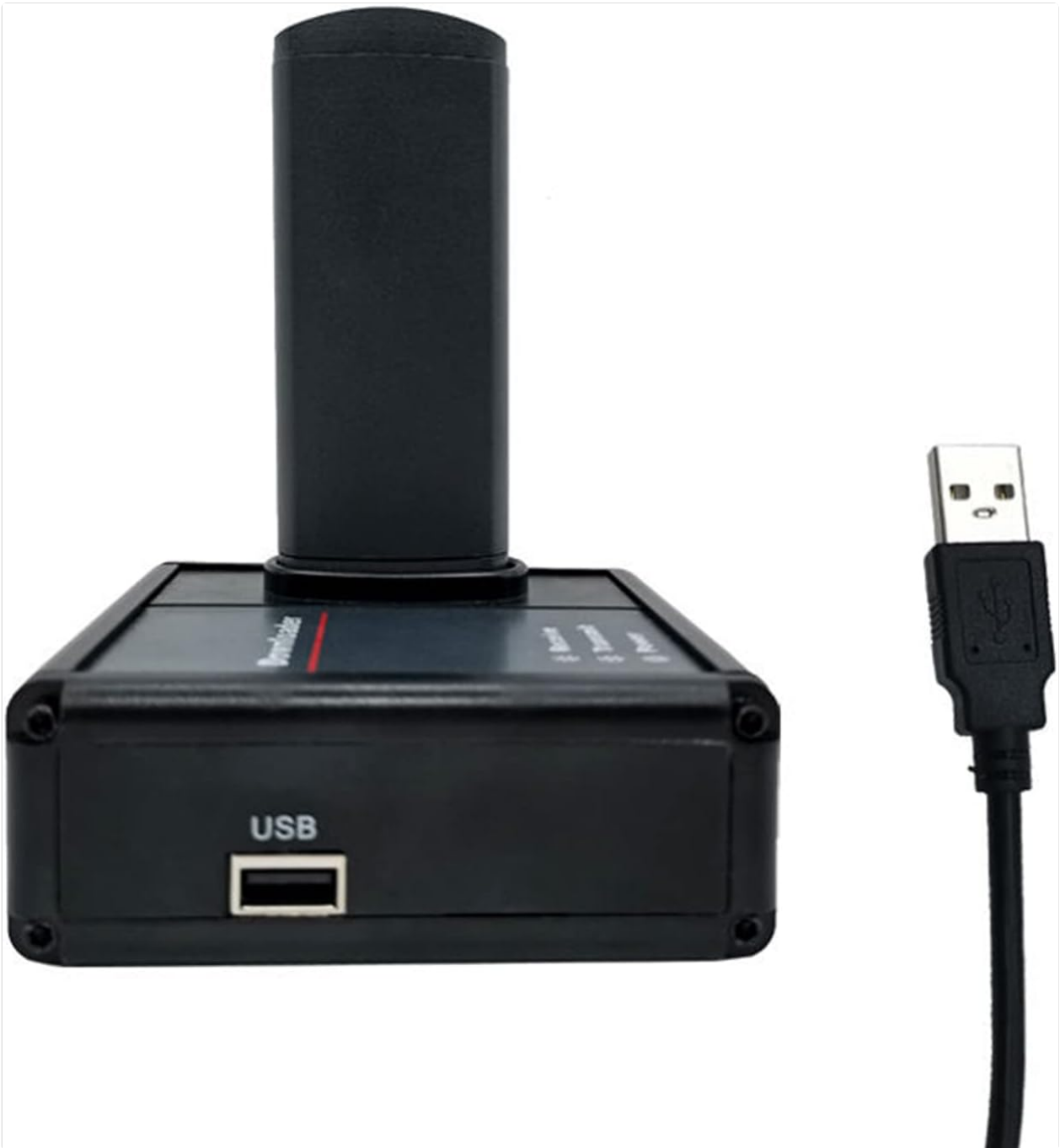
Figure 4: The data downloader connected to a computer via USB cable, ready for software interaction.
