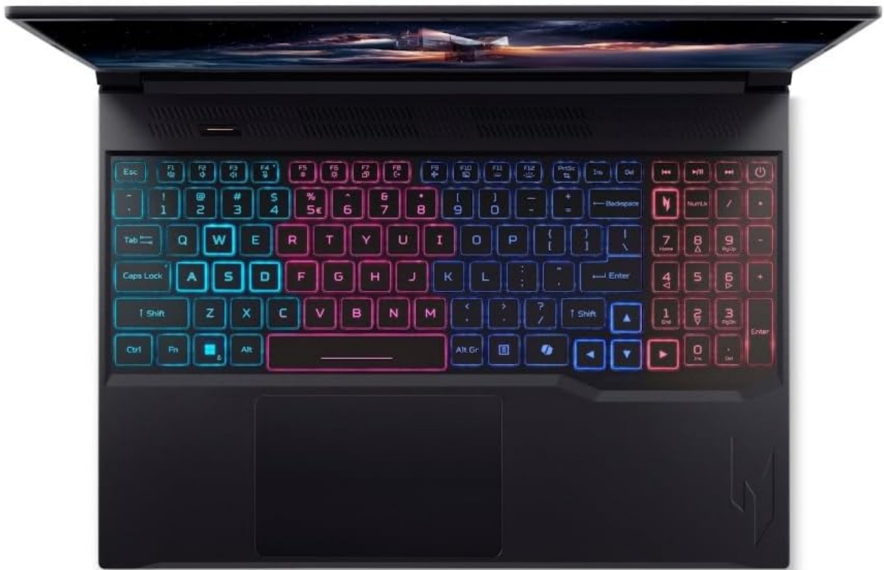
Figure 2.3: Top-down view of the Acer Nitro V 16 Slim laptop's keyboard, featuring multi-zone RGB backlighting and a full numeric keypad.
