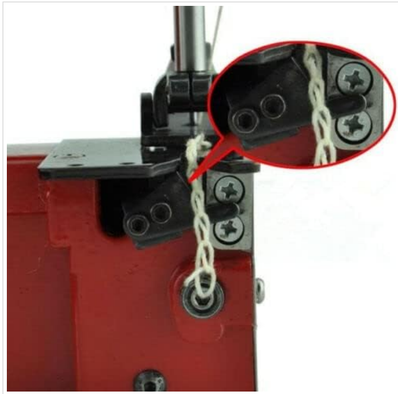
Figure 4.1: Close-up view illustrating the threading path for the GK9-350 sewing machine. The image highlights how the thread passes through tension discs and guides to form a secure chain stitch, with an inset showing the final stitch formation.
