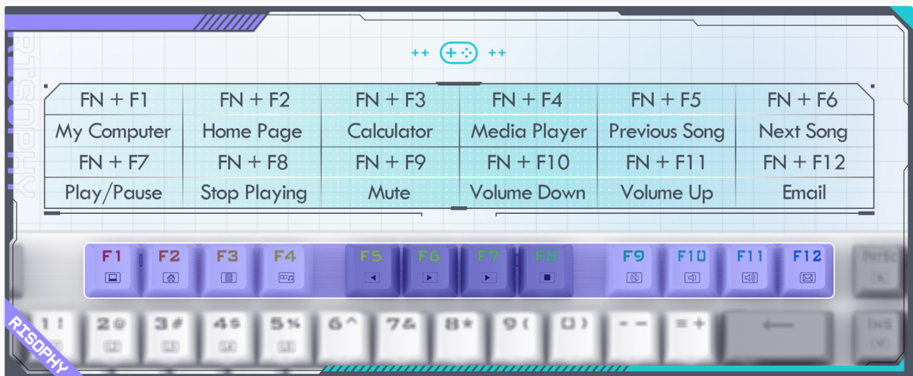
Image: A visual guide to the FN key combinations (F1-F12) and their corresponding multimedia and system functions.
