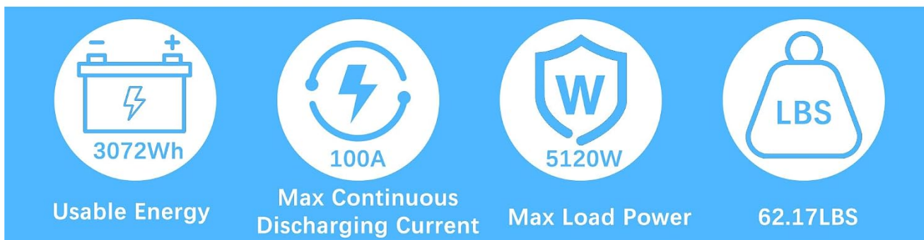
Figure 3.2: Key dimensions and specifications of the OCELL 48V 60Ah LiFePO4 Battery.
