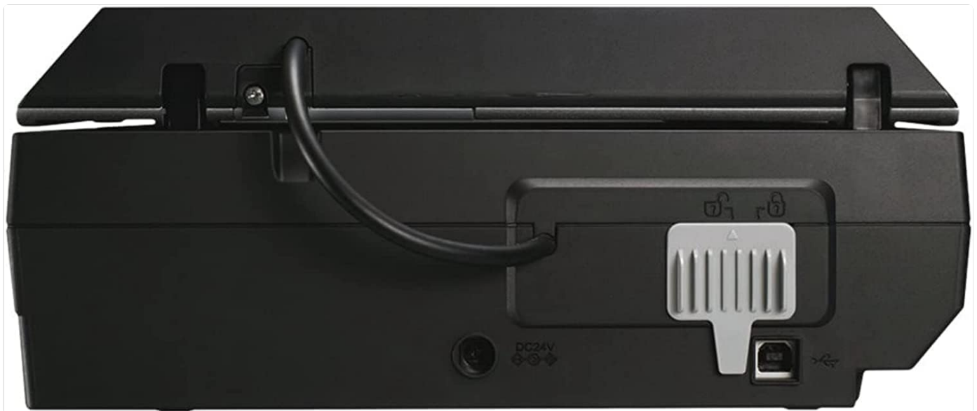
Figure 4: Rear view of the scanner, highlighting the DC24V power input and the Hi-Speed USB 2.0 port for connection to a computer.
