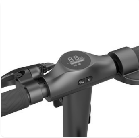
Image 3.3: Handlebar with integrated LED display.
