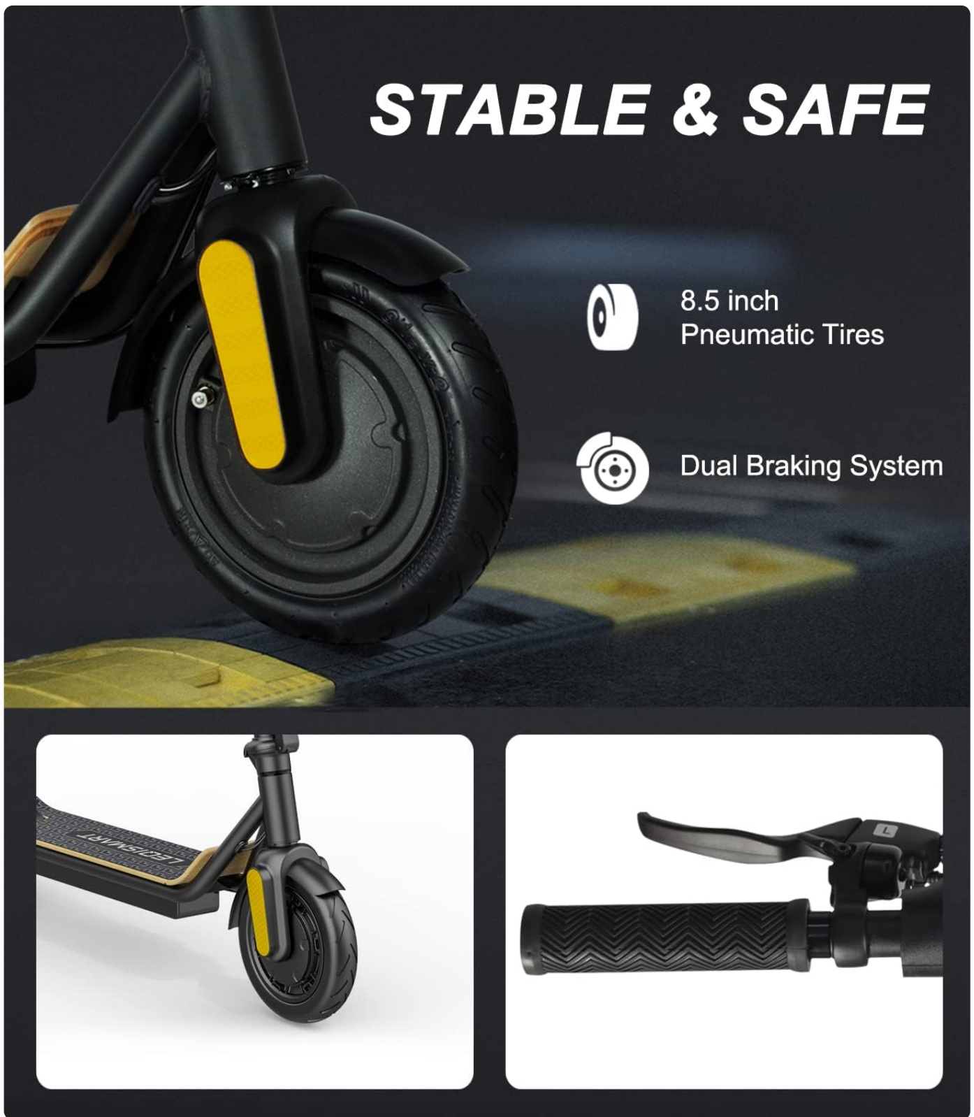
Image 2.1: Detail of the 8.5-inch pneumatic tires and the dual braking system, highlighting safety features.
