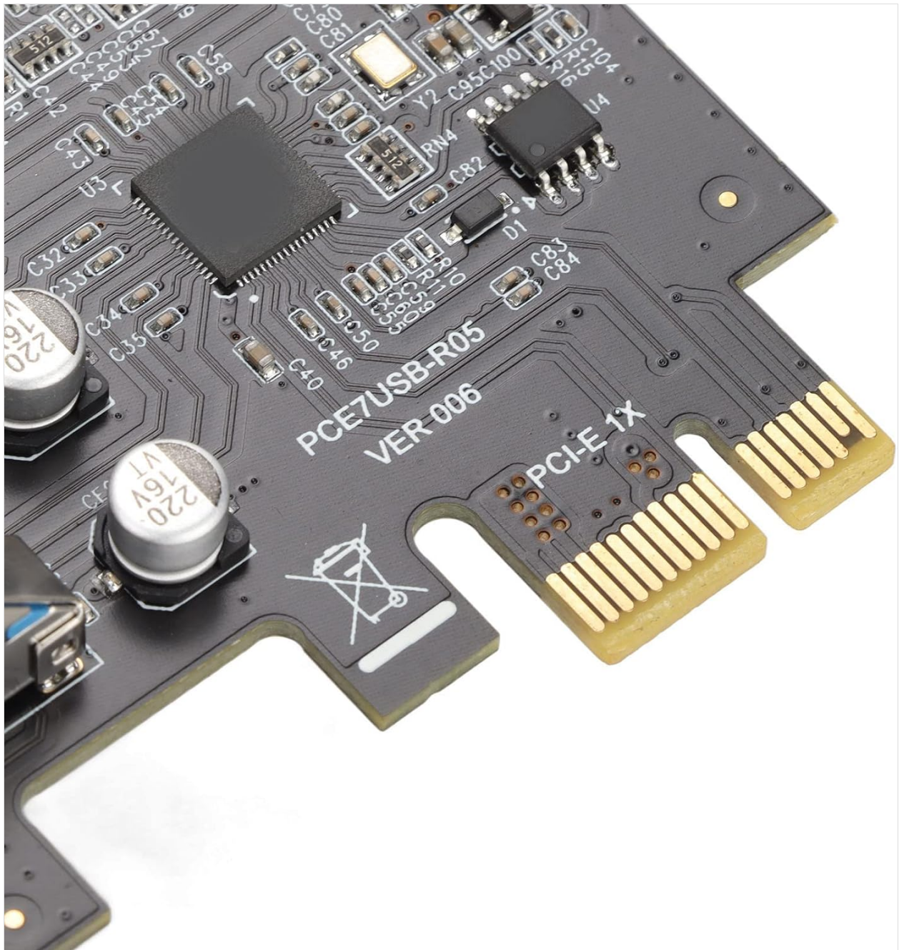
Figure 3.1: Close-up view of the PCIe x1 connector on the expansion card.
