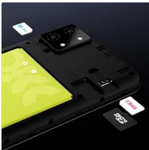
Image: Internal view of the NUU A9L, highlighting the battery, SIM, and microSD card slots.
