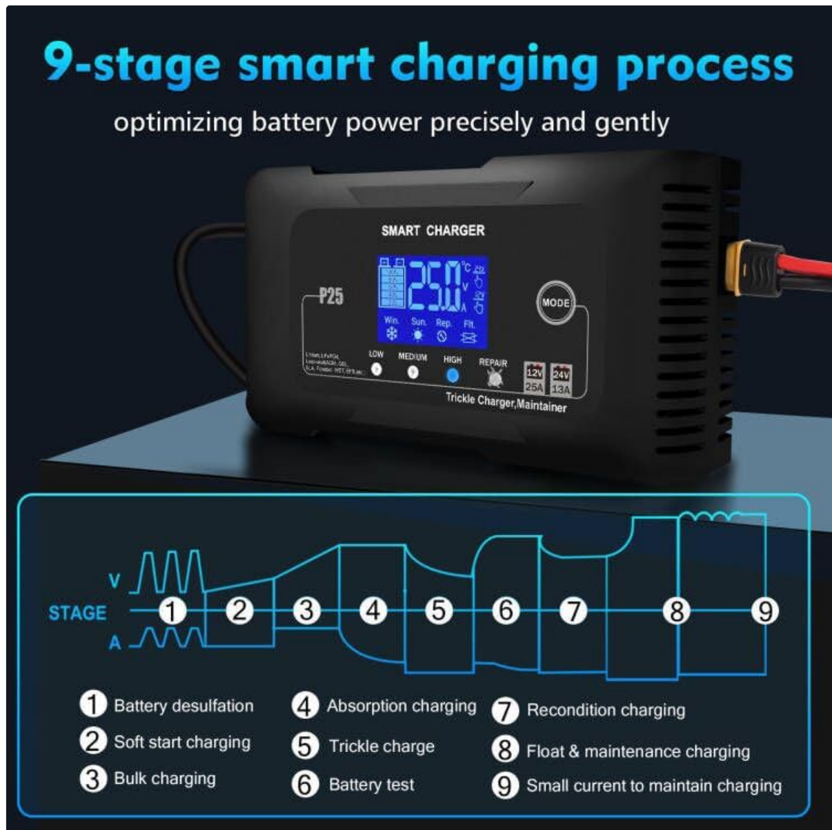
Figure 5.2: Detailed diagram of the 9-stage smart charging process.
