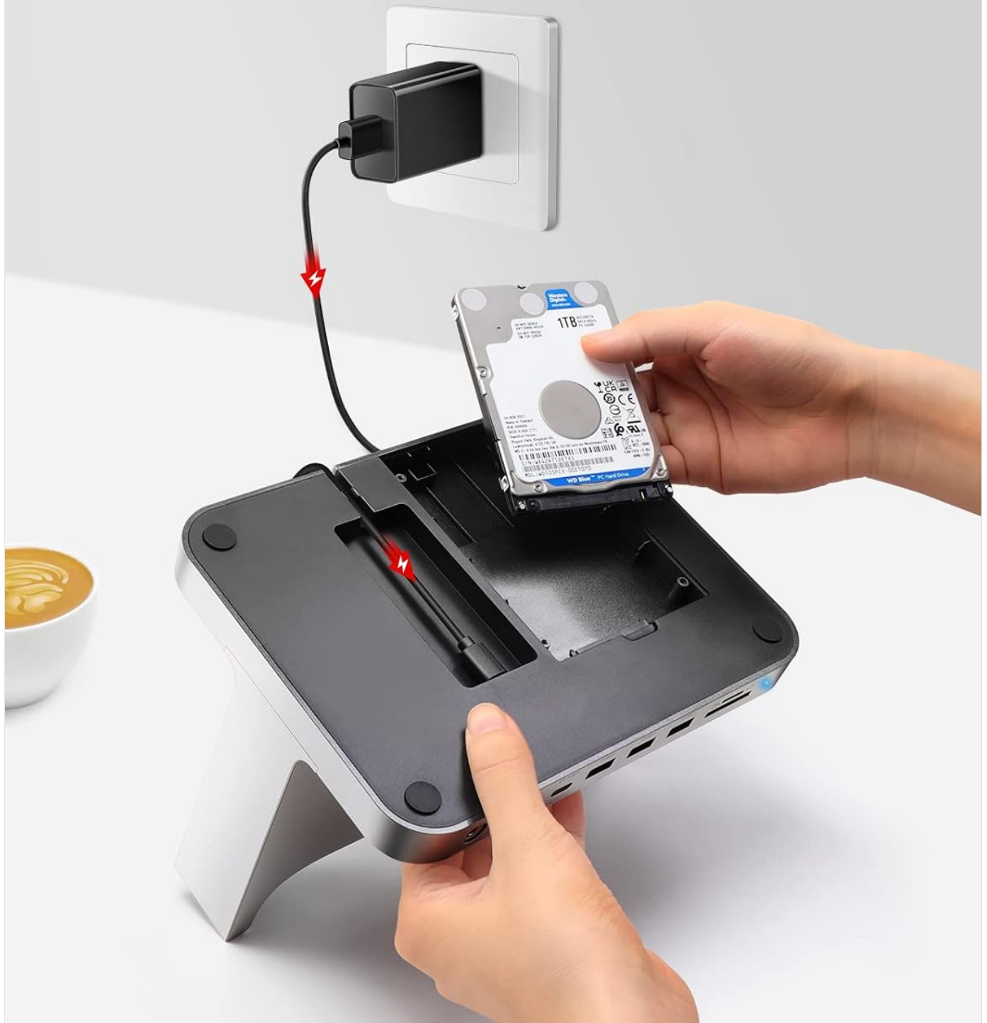
Image 3.2: Step-by-step guide showing the installation of a 2.5-inch HDD/SSD into the dedicated bay at the bottom of the VAYDEER Mac Mini Stand, and
