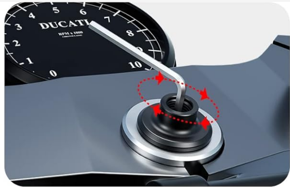
2 Tighten the base with an Allen Wrench
