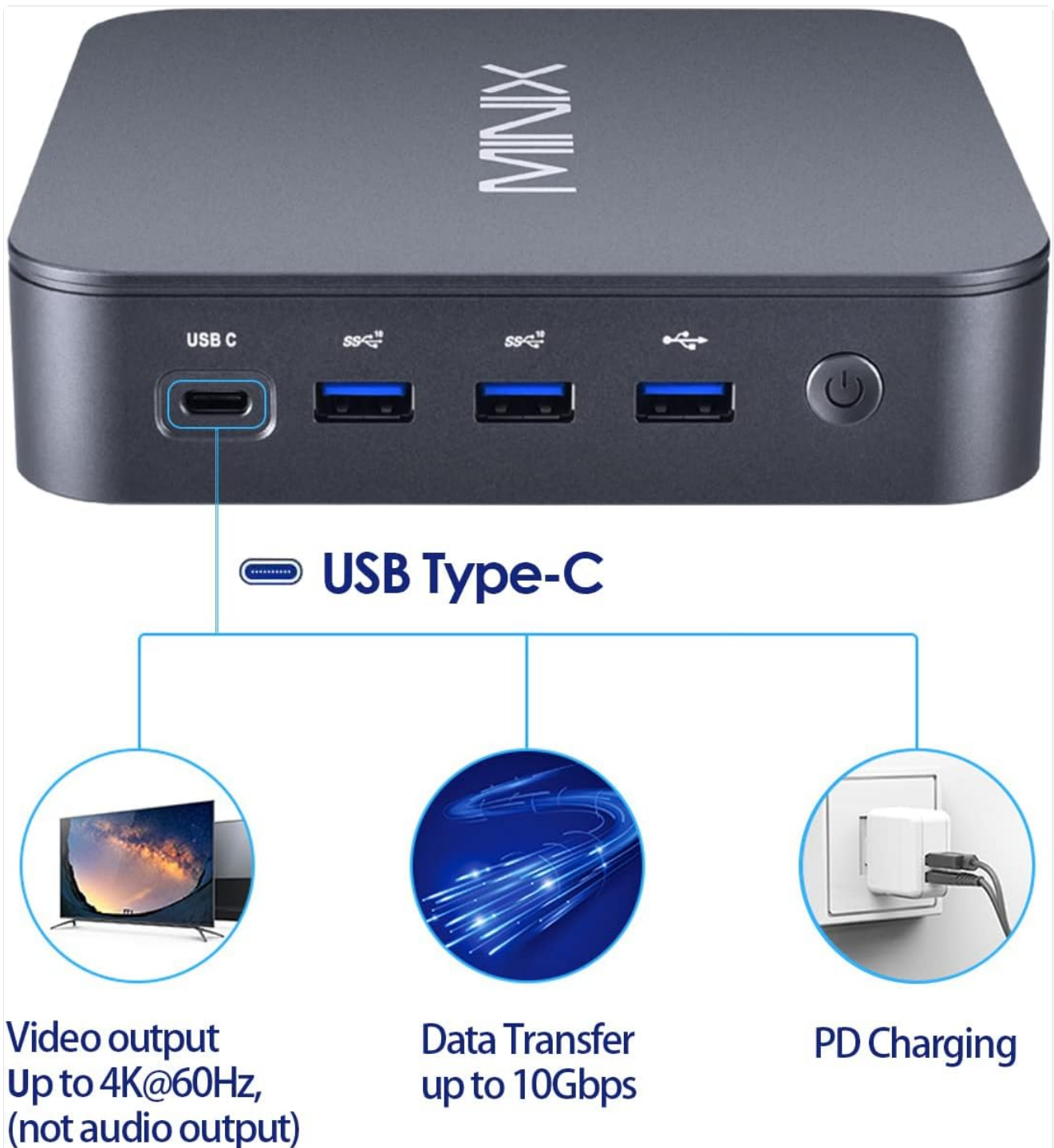
Figure 3: USB Type-C Port Functionality. This image highlights the versatility of the USB-C port, supporting video output up to 4K@60Hz (no audio output), data transfer up to 10Gbps, and PD Charging.
