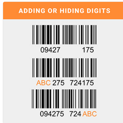
Image: Example of adding or hiding digits in scanned barcode output.
