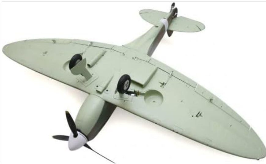
Figure 3: Underside view of the Duraflly Spitfire Mk2a, highlighting the retractable landing gear in the extended position and the overall wing structure.
