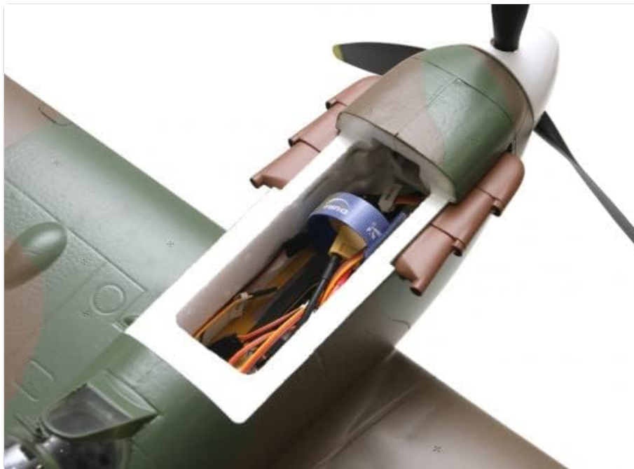
Figure 2: Close-up view of the battery and receiver compartment located in the nose section of the Duraflly Spitfire Mk2a, showing ample space for component installation.
