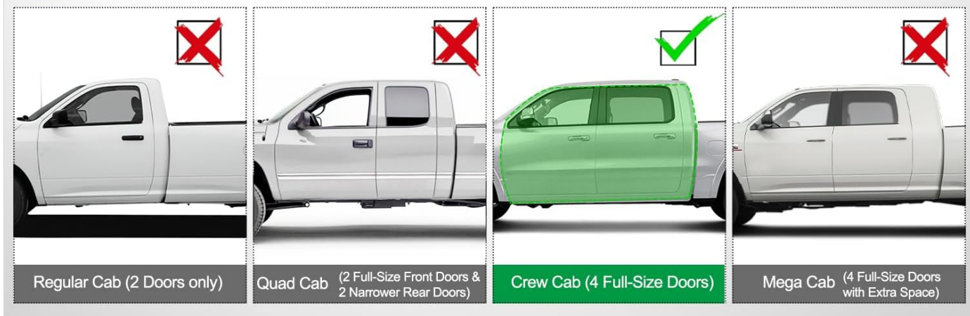
Figure 2: Vehicle Fitment Type. This diagram helps identify the correct cab type for installation, highlighting that the running boards are compatible with Crew Cab models.
