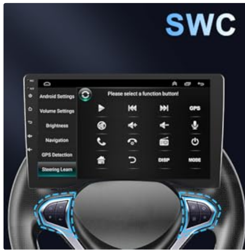
Image 3.9: The car stereo's settings menu for Steering Wheel Control (SWC), showing how to map vehicle steering wheel buttons to stereo functions.
