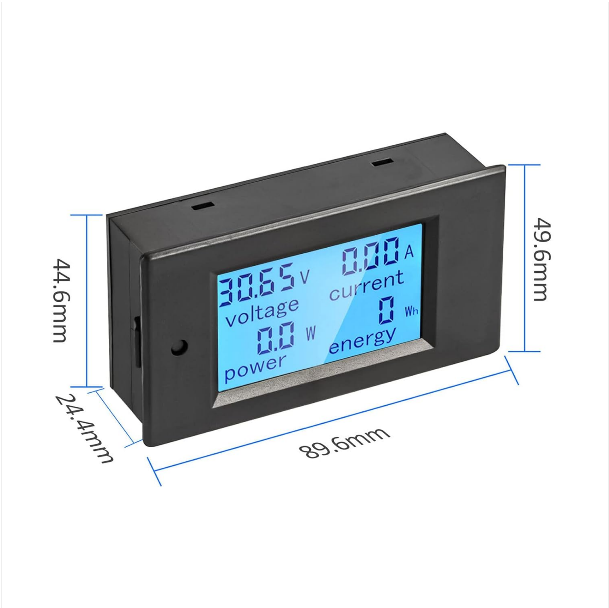
Figure 1: Voktta 100A DC Power Meter with labeled dimensions (89.6mm x 44.6mm x 24.4mm).
