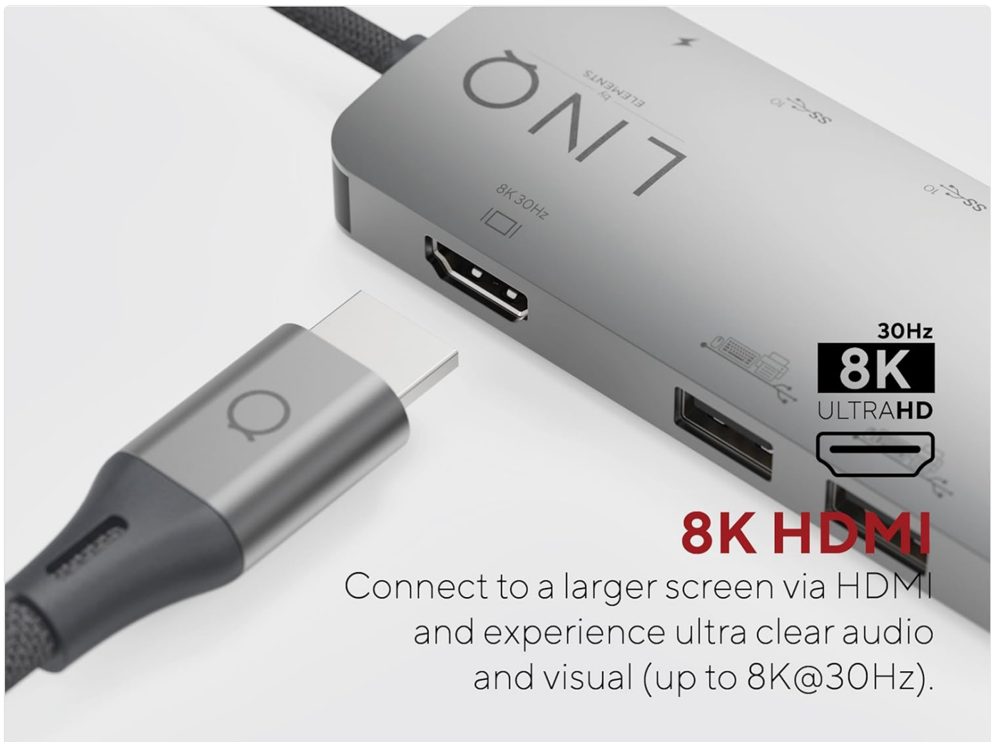
Image: Close-up of the 8K HDMI port on the LINQ Hub, highlighting its high-definition video output capability.
