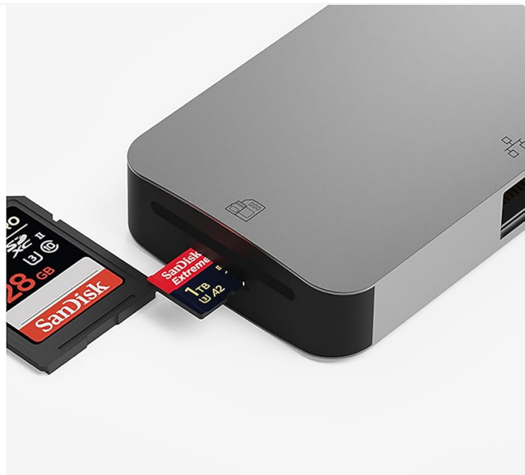
Figure 4: The UHS-II SD 4.0 Card Reader for high-speed memory card access.
