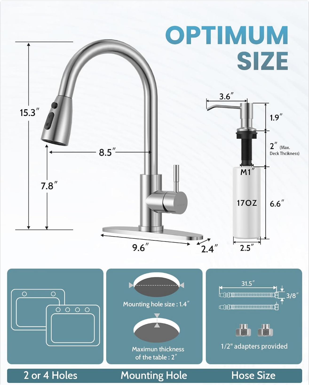
Figure 13: Optimum dimensions and installation requirements.
