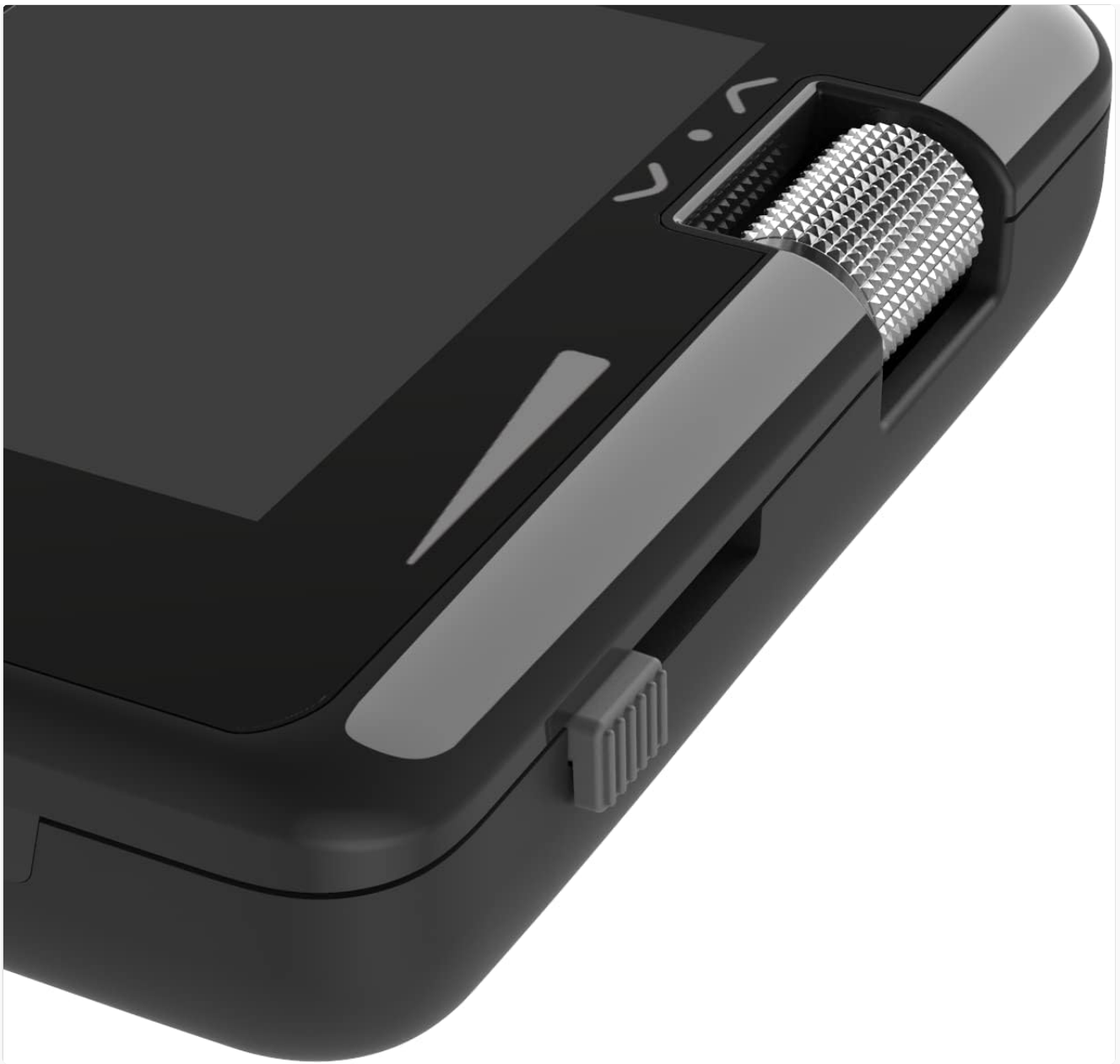
Figure 5: The metal roller and slider provide precise control.
