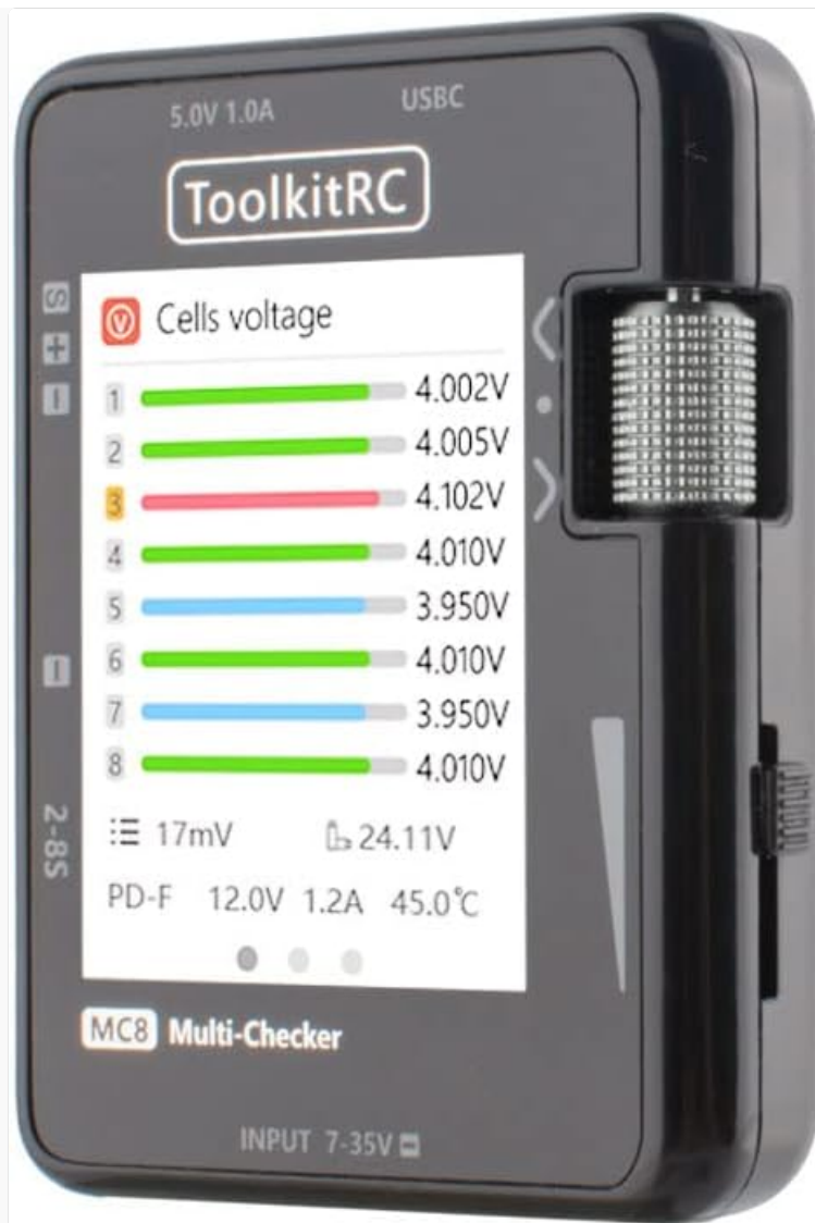
Figure 6: The display shows detailed cell voltage information.
