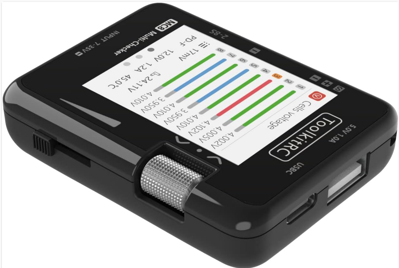
Figure 7: USB-A and USB-C ports for charging and firmware updates.
