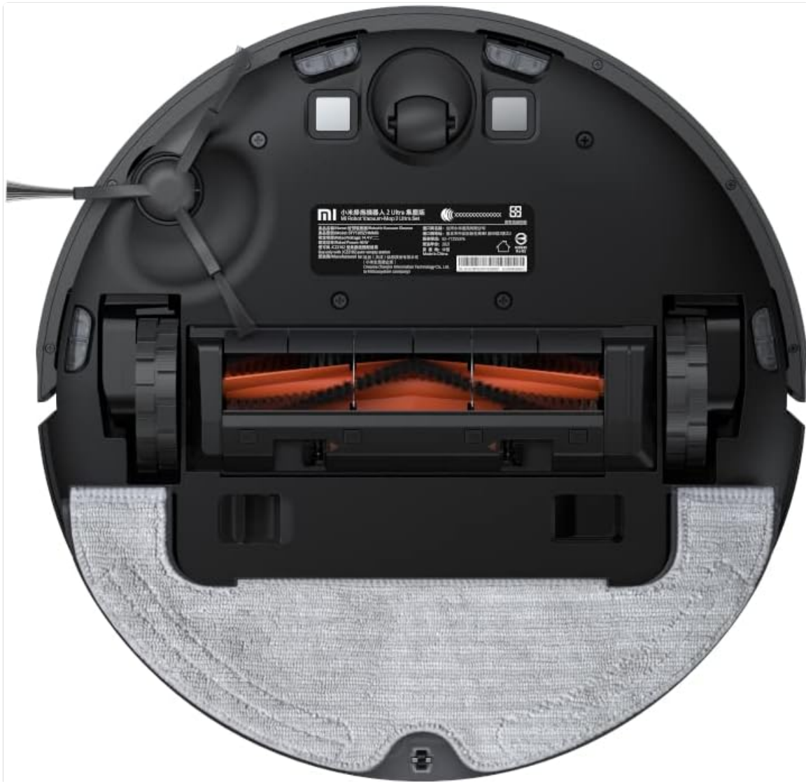
Image: The underside of the Xiaomi Vacuum-Mop 2 Ultra, displaying the main brush, side brush, and attached mop pad, indicating areas for maintenance.
