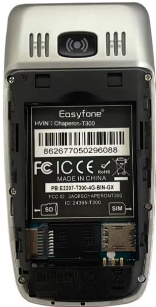
Image: Rear view of the Easyfone T300, showing the internal battery compartment and slots for SIM and SD cards.
