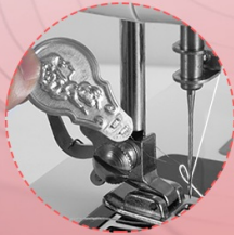
Image: Visual guide emphasizing threading the needle from front to back to prevent thread breakage.
