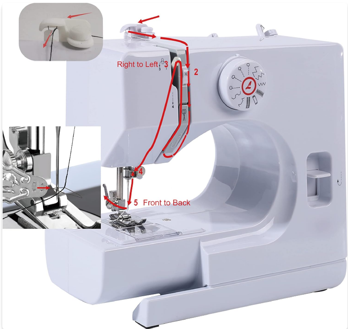
Image: Detailed diagram illustrating the correct path for threading the upper thread.
