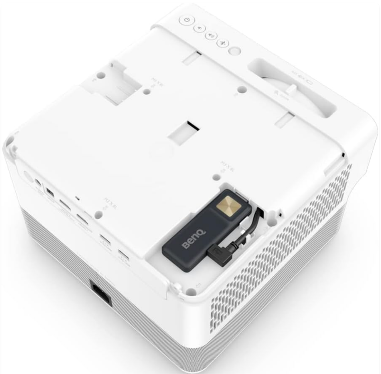
Figure 5: Location of the internal Android TV dongle slot.
