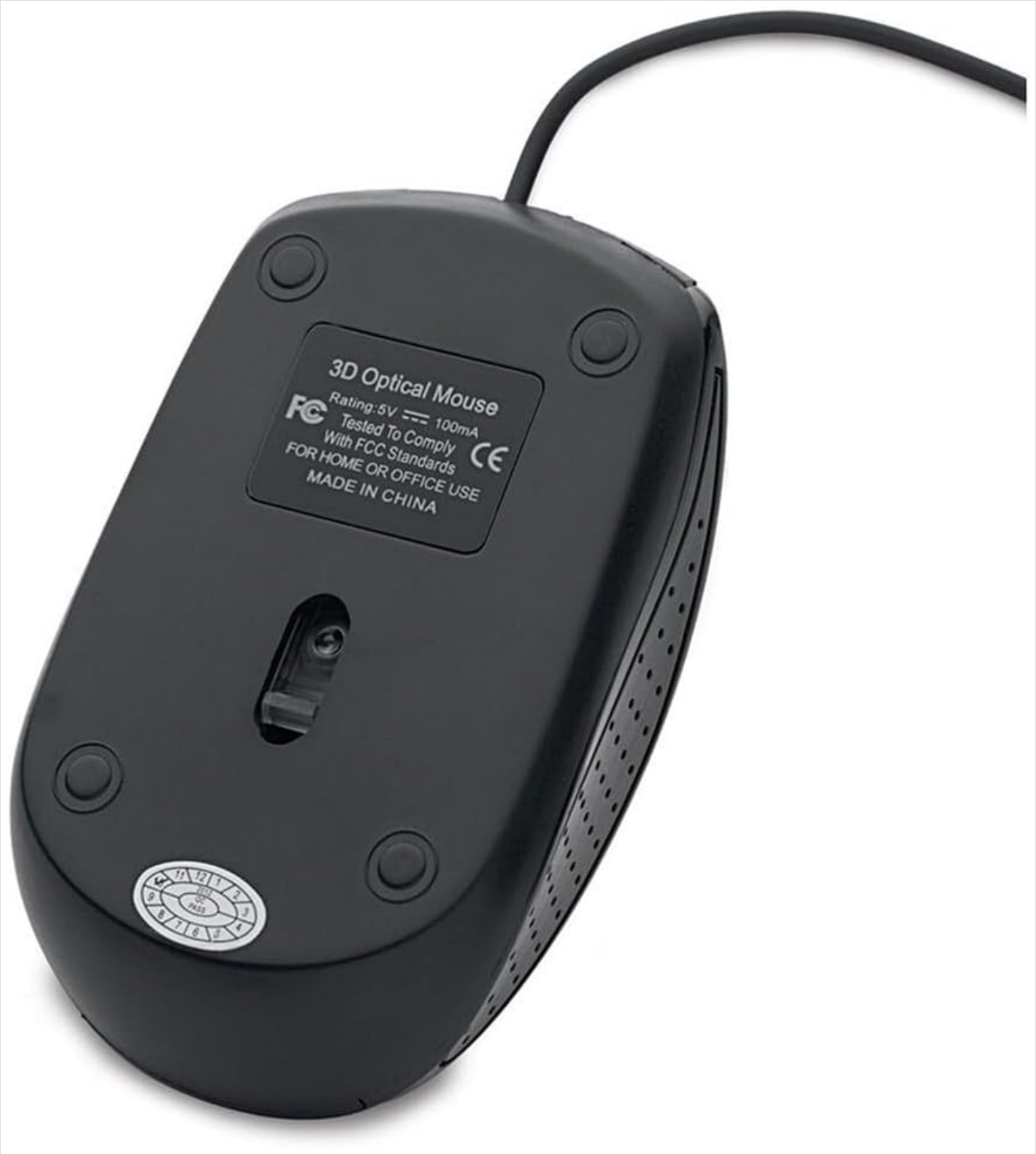
Image 5.1: Underside view of the Verbatim 70733 mouse, showing the optical sensor and product labeling.
