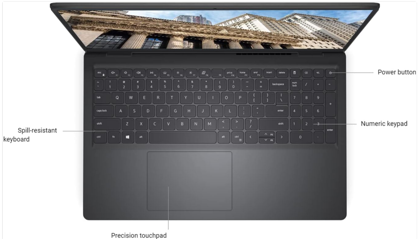
Figure 3: Top-down view of the Dell Vostro 3520 laptop, illustrating the keyboard, precision touchpad, power button, and numeric keypad.
