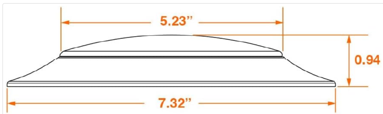
Figure 2: Product Dimensions. The light disk measures 7.32 inches in diameter and 0.94 inches in height.
