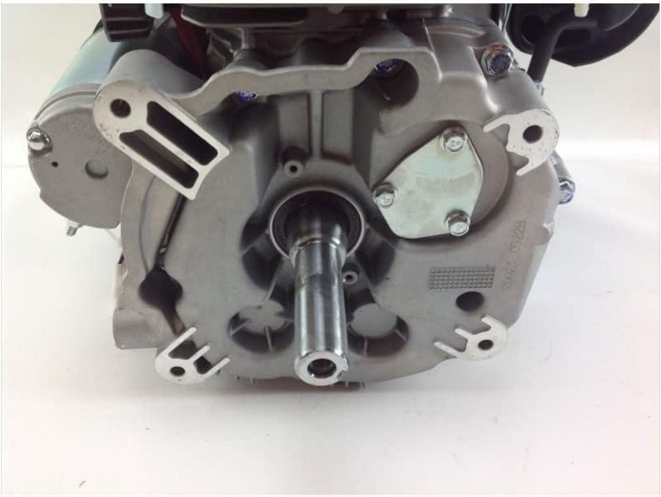
Figure 3.2: Bottom view of the engine, highlighting the crankshaft for connection to the drive system.
