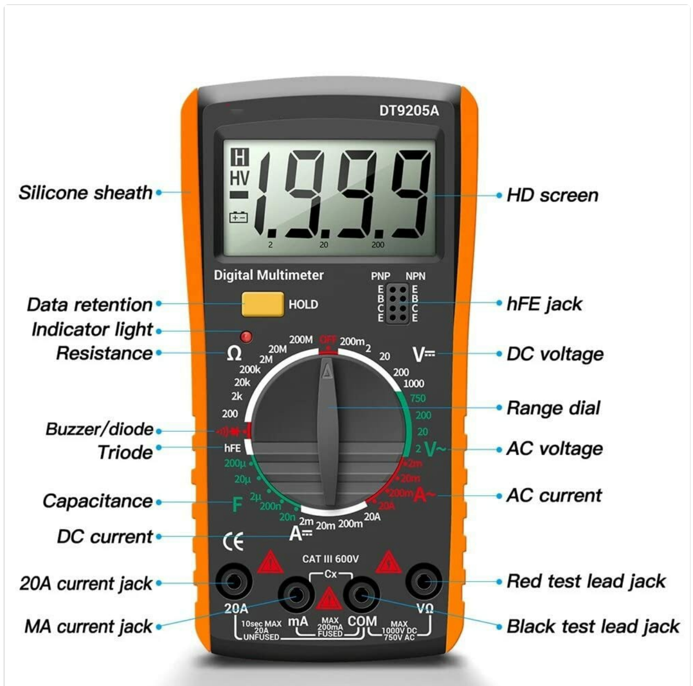
Figure 1: DT9205A Multimeter Front Panel Layout
