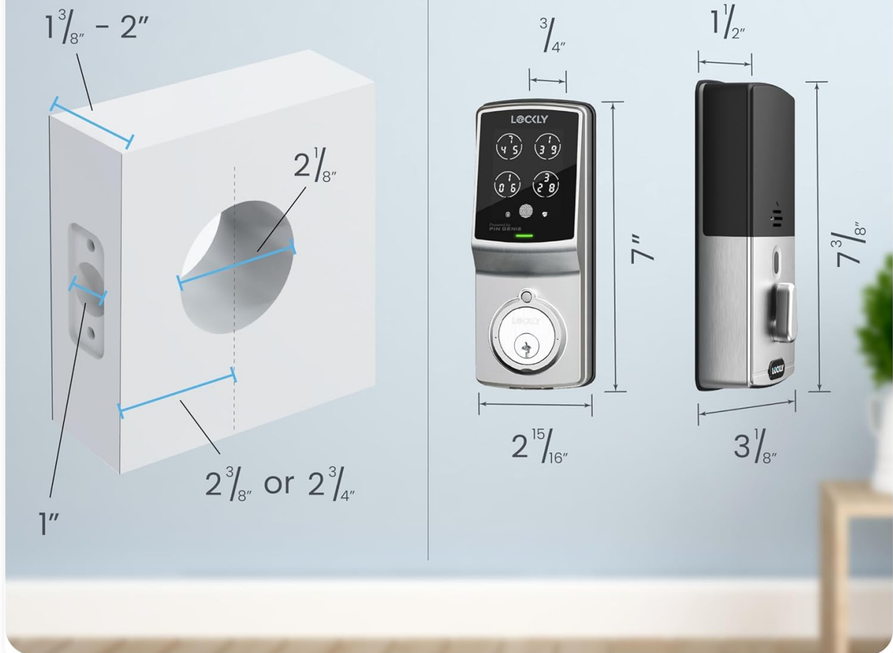
Figure 2: Door compatibility diagram illustrating required measurements for installation.
