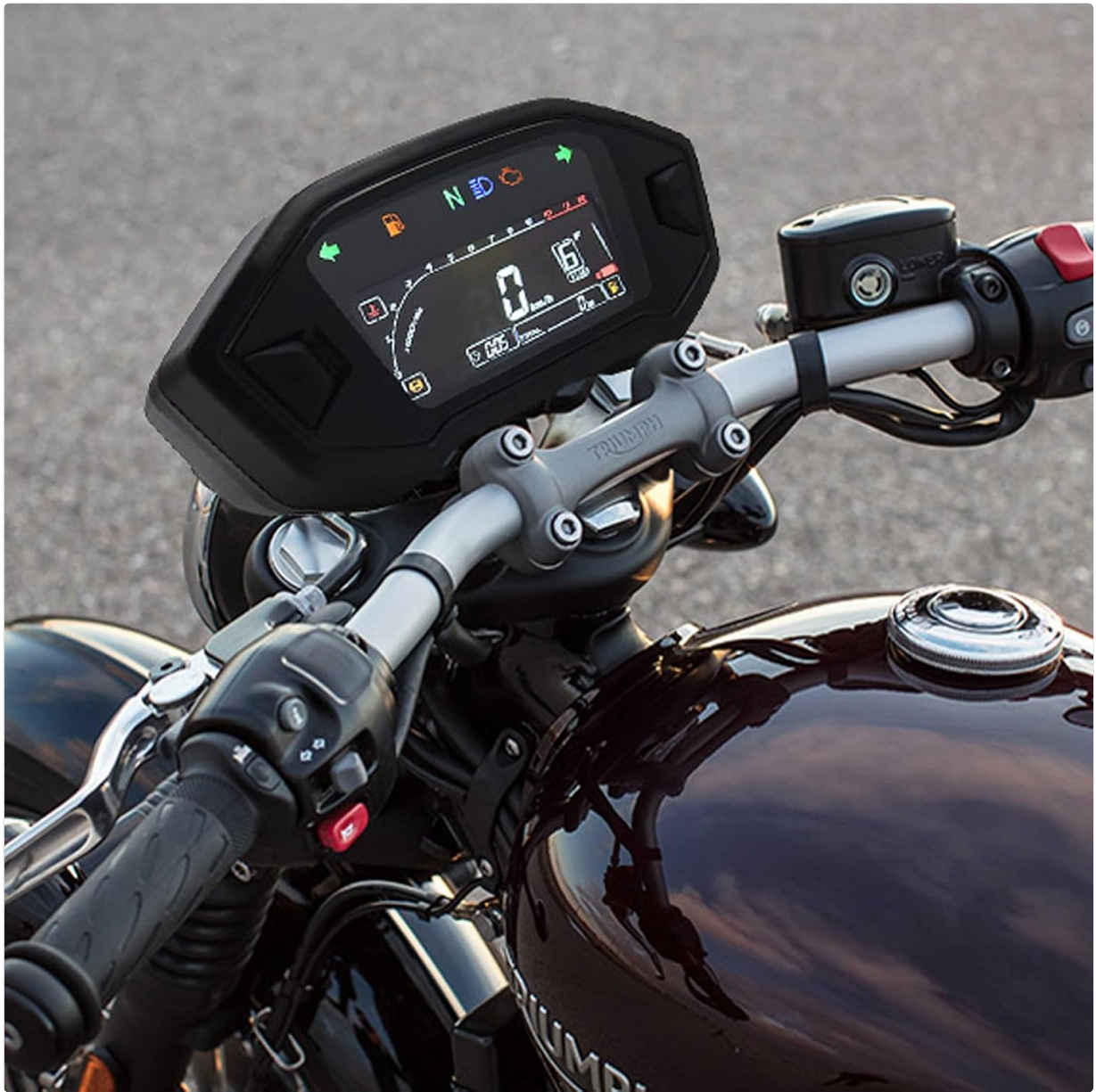
Image 5.1: Example of the tachometer installed on a motorcycle handlebar.
