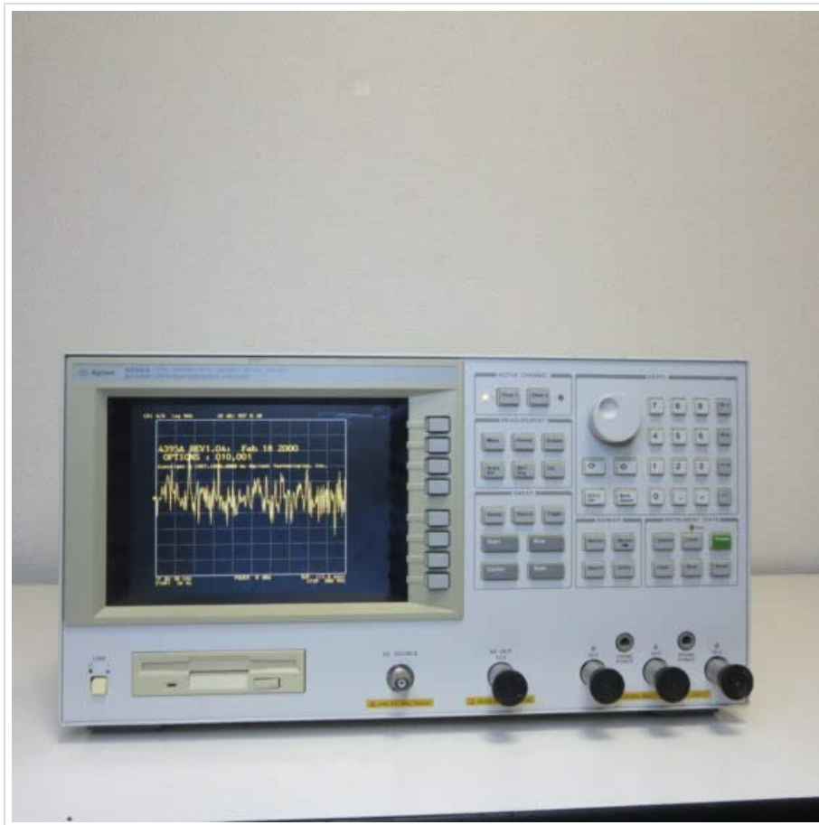
Figure 2.1: Front view of the Keysight 4395A Network/Spectrum/Impedance Analyzer, showing the display, floppy drive, and control buttons.
