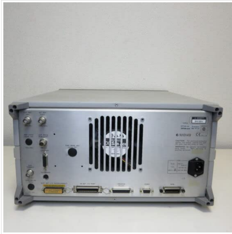
Figure 2.3: Rear view of the Keysight 4395A, detailing power input, GPIB, and other connectivity ports.
