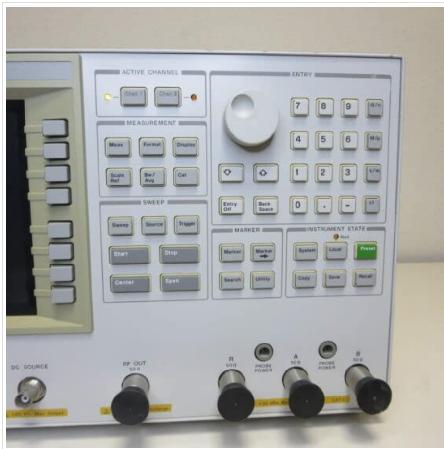
Figure 2.4: Close-up of the Keysight 4395A control panel, showing the rotary knob, numeric keypad, and function buttons for measurement and display settings.
