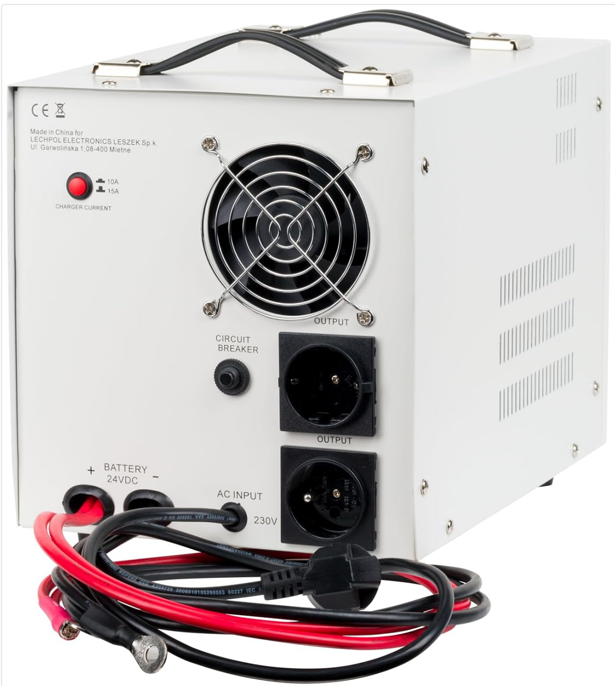
Figure 2: Rear view of the Kemot PROsinus-2000 inverter. This image shows the back of the inverter, highlighting the 24V DC battery input terminals (red for positive, black for negative), the 230V AC input socket, two 230V AC output sockets, a circuit breaker, and a cooling fan. The charger current settings (10A/15A) are also visible.
