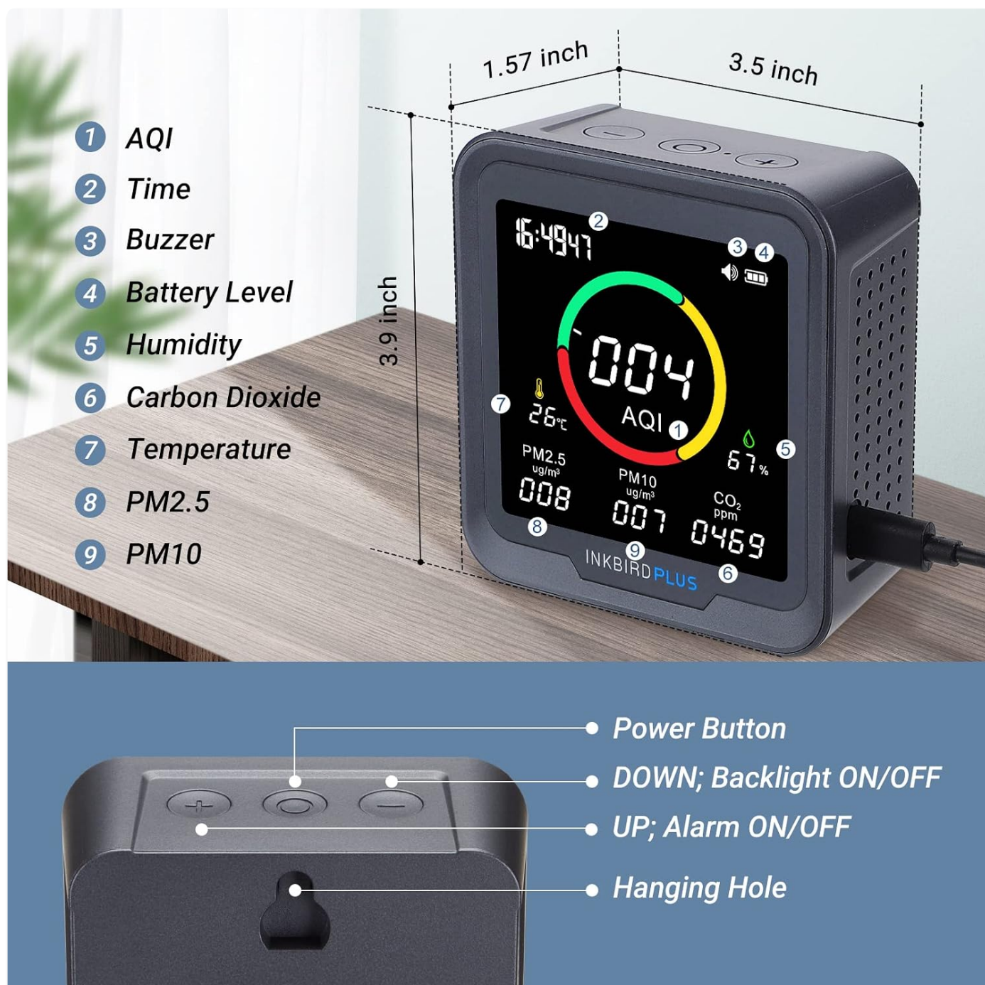
Figure 1: Front and side view of the INKBIRDPLUS PTH-9A with labeled components and dimensions.
