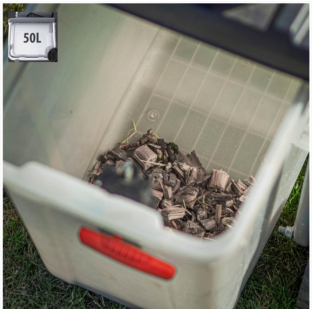
Figure 4.3: The transparent 50-liter collection bin, showing processed wood chips. The bin's capacity is indicated.
