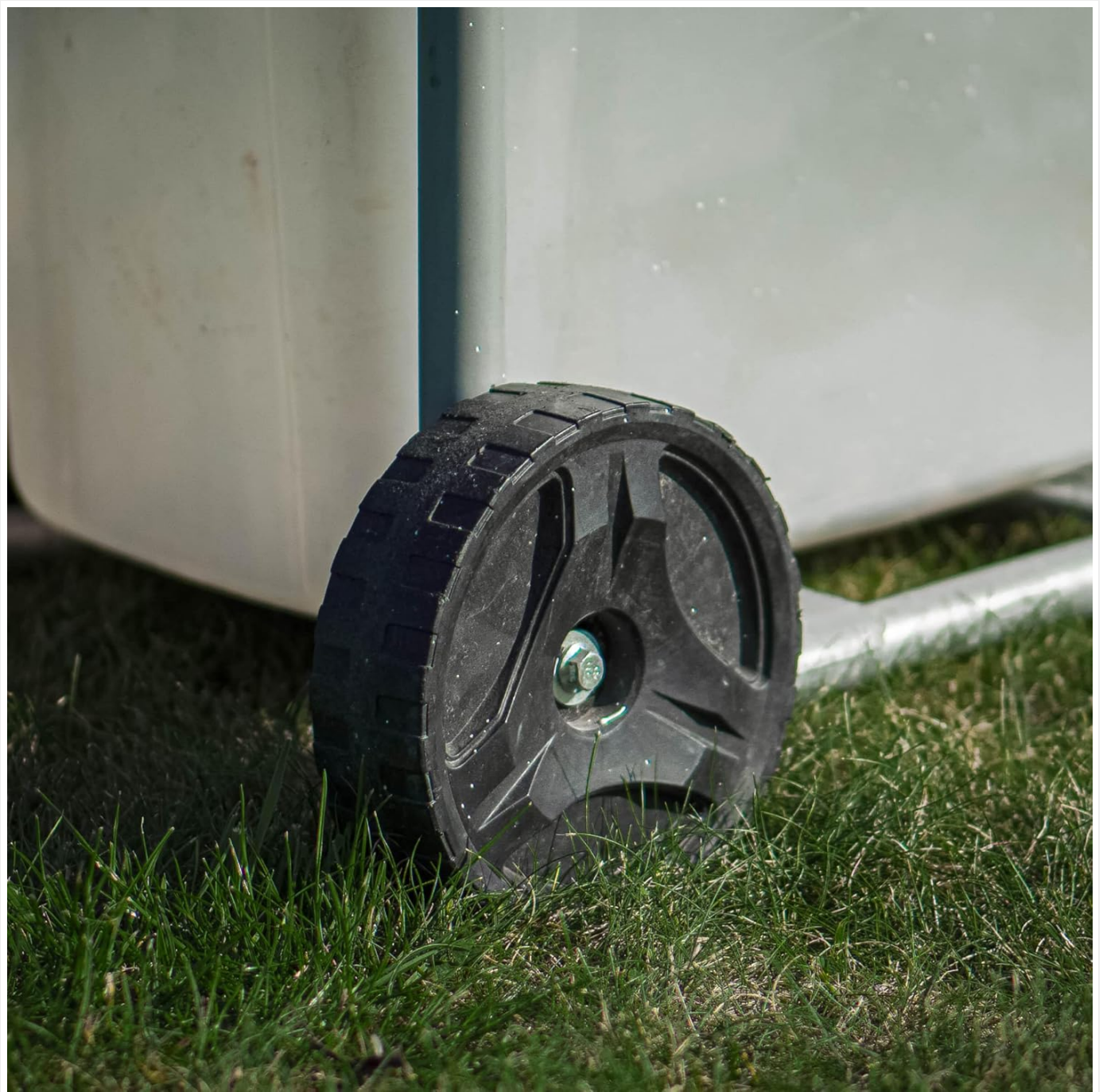
Figure 3.1: Detail of one of the wide wheels, highlighting the shredder's portability features.
