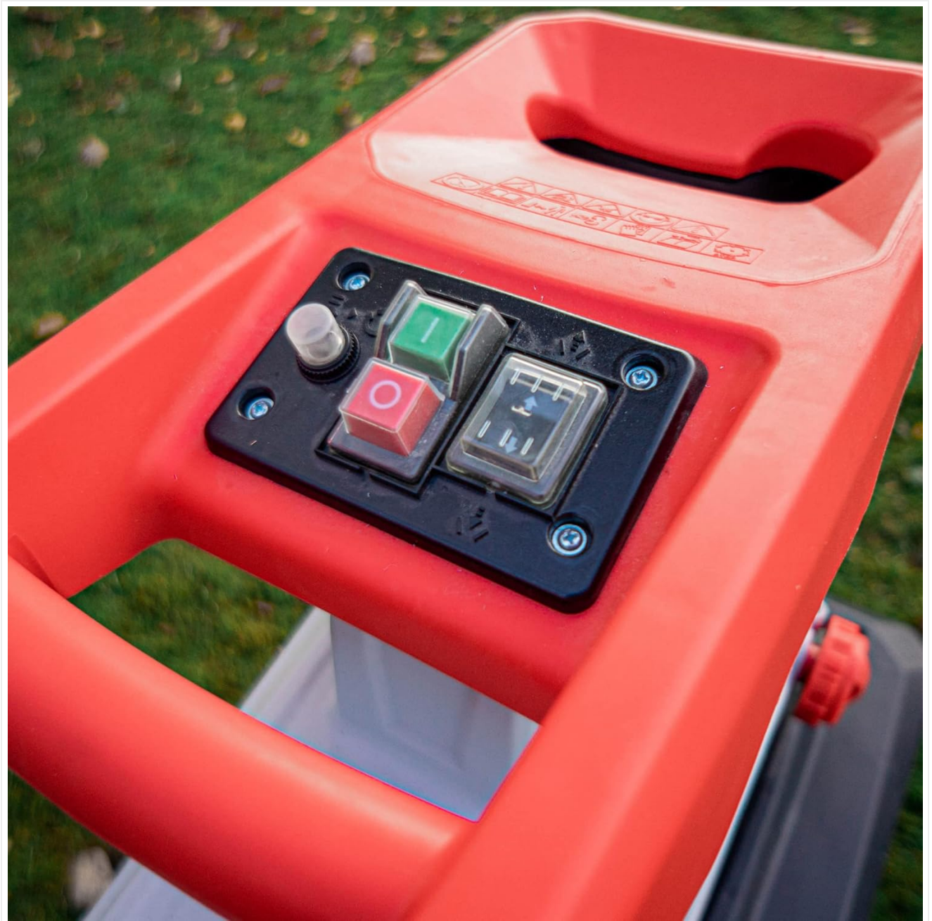
Figure 4.2: The control panel showing the green start button, red stop button, and the reverse switch for clearing jams.
